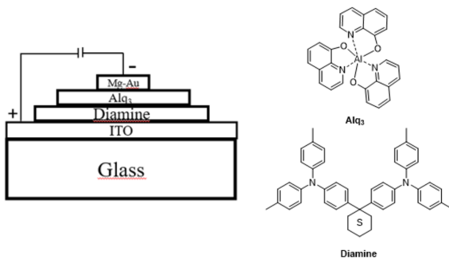
Figure 1.7. The first electroluminescence in organic structures device architecture
